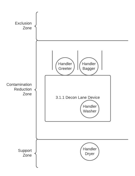
**Decon Lane Layout:** The Contamination Reduction Zone can be arranged to meet the overall incident objectives and leader's intent of the incident commander. Handlers assigned to Decon Lane Manager fill the functions as needed. Ambulatory and non-ambulatory patients are greeted and moved through the decon lane device.
